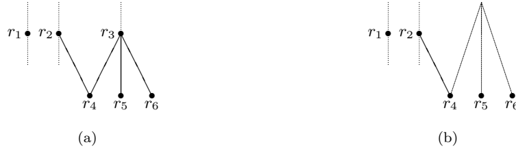
Fig. 7. Role deletion and SARBAC constraints: If r_3 is deleted then the constraint r_1 \wedge r_2 \wedge r_3 is replaced by \bigwedge \{r_1, r_2, r_4, r_5, r_6\} = r_1 \wedge r_2 \wedge r_5 \wedge r_6
