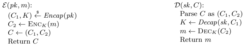
Fig. 3. Construction of a public-key encryption scheme from a KEM and a DEM
